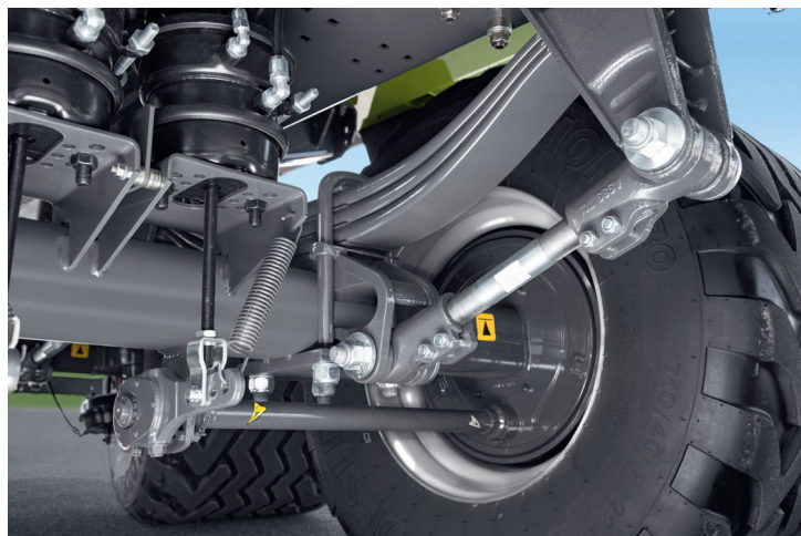
Mechanical parabolic suspension, as standard with spring travel limiter bushes for maximum stability
