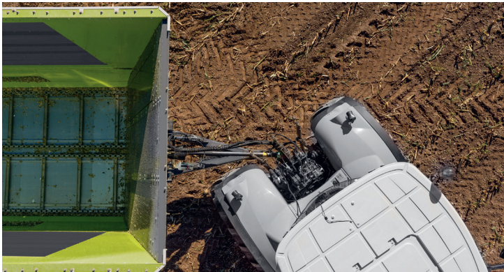
Extremely slim design for maximum steering angle
