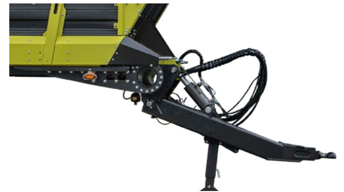
CARGOS 700 dissel, disselbelasting 3 of 4 ton
