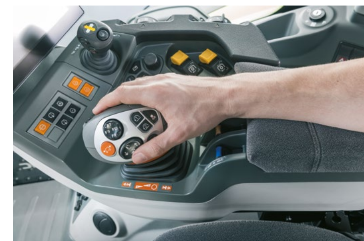
Programming the ISOBUS functions on the JoyStick
