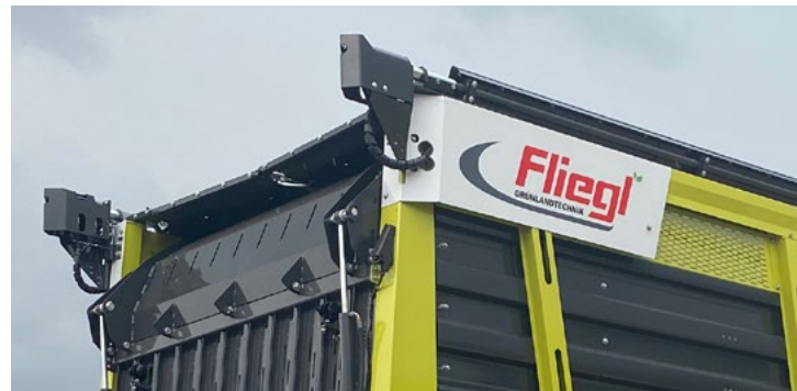
Pressure measurement on the filling flap and torque sensor on the rotor. This combination of both sensors guarantees optimum filling of the wagon and full utilisation of the loading volume.
