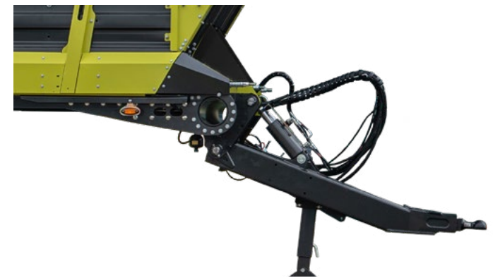
CARGOS 700 drawbar, drawbar load 3 or 4 tonnes
