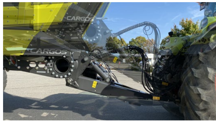
Articulated drawbar á la Sytem lift axle
