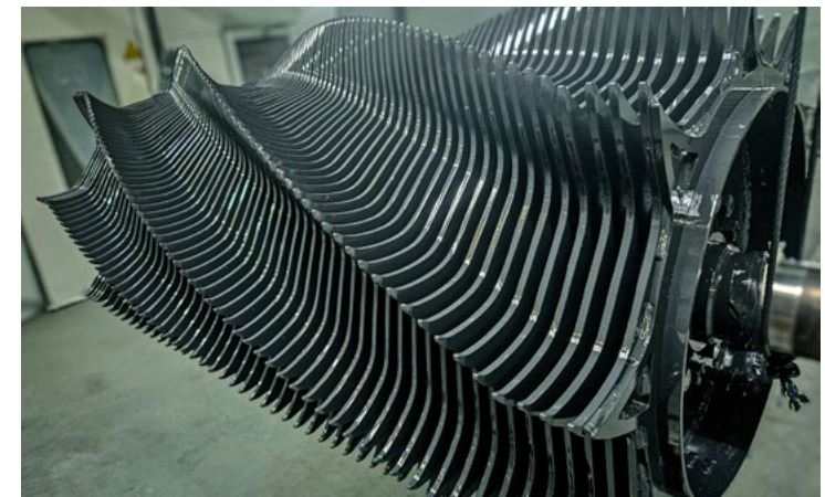
Nine rows of rotor tines mounted and welded onto the rotor shell
