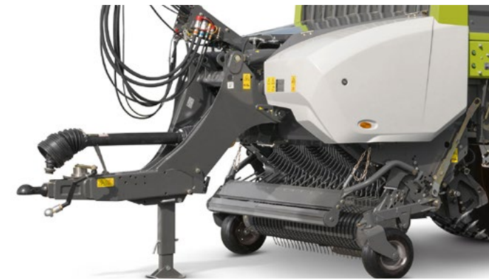
Drawbar CARGOS 8000/9000, drawbar load 3 or 4 tonnes
