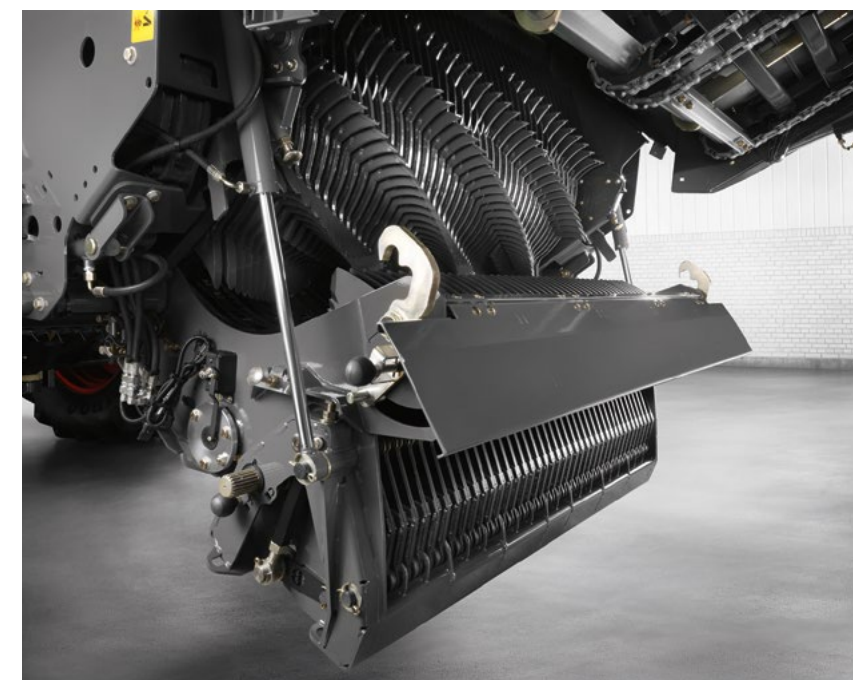
Free access to the rotor in the cleaning position.
