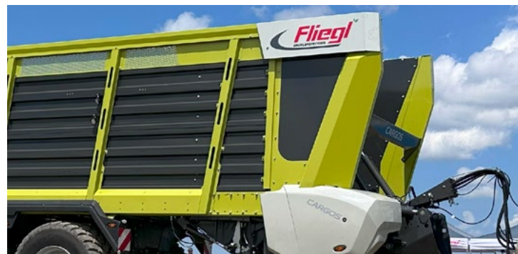
Swivelling front wall Pro, hydraulically swivelling - for even more loading volume and faster unloading.
