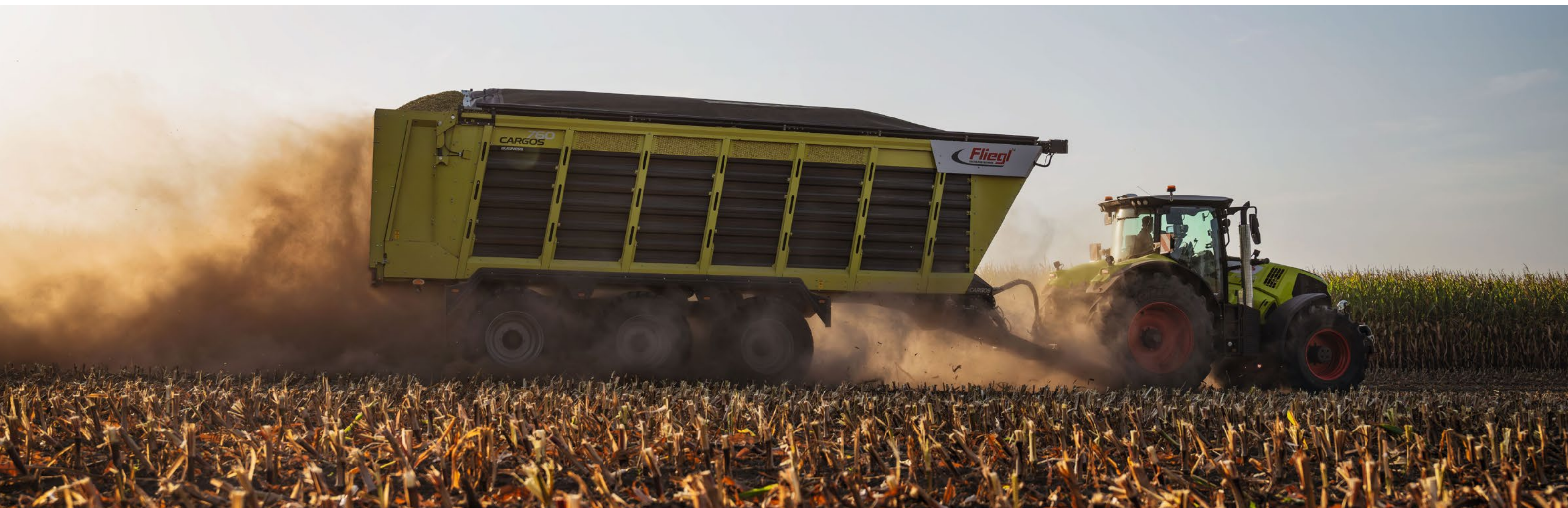
Drawbar CARGOS 8000/9000, drawbar load 3 or 4 tonnes
