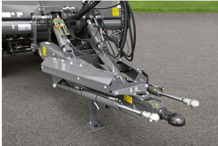
Mechanical-hydraulic forced steering tridem vehicle
