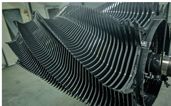
Nine rows of rotor tines mounted and welded onto the rotor shell
