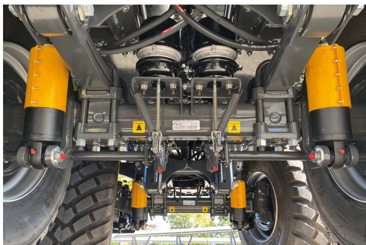
Hydraulically sprung running gear with automatic slope levelling
