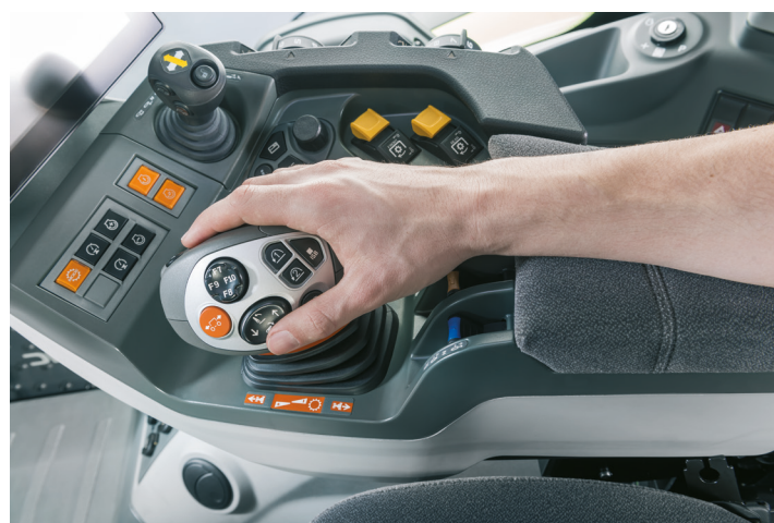
Programming the ISOBUS functions on the JoyStick
