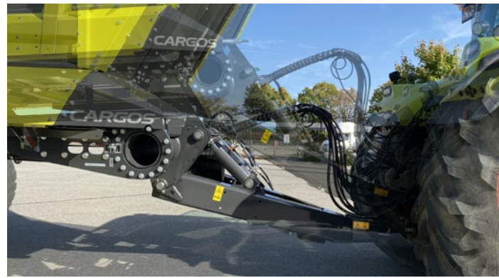
Knickdeichsel á la System Liftachse
