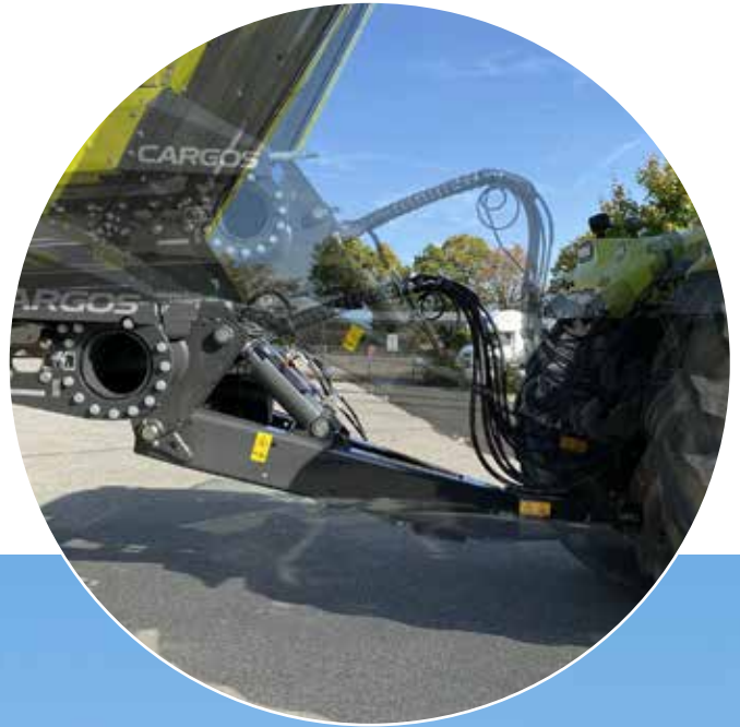
Extremely slim design for maximum steering angle
